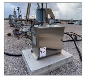
manages annular pressure so that more free gas stays in solution. This increases the oil's mobility and eliminates, or largely eliminates, gas interference in the pump. Gasification & gas lock are a problem on any well, but especially in pumps on unconventional wells.
